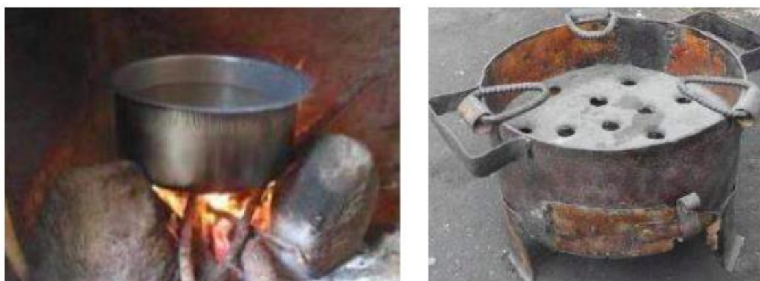
Figure 1: Traditional stoves used in Tanzania (Left: Three stone fire, Right: single walled metal charcoal stove)
